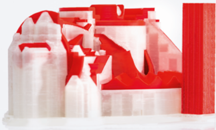
Model of gear mechanism before support material dissolution
